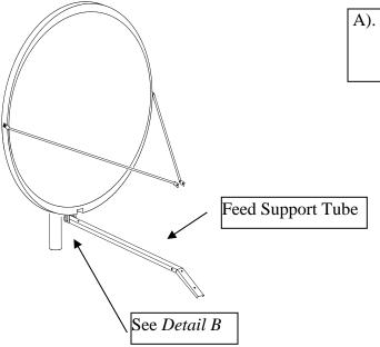
A). Mount feed support tube between the feed support brackets with [2] of (items: 8, 5, 6, 7).
